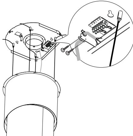
Finally, check that the power supply cable is properly locked, checking that when the mobile unit rises up towards the ceiling, it positions itself over the mobile unit and does not come out from the edge of the hood.
