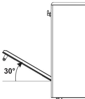
3. To reassemble the door, put the hinges in the relevant slots in the oven, making sure that grooved sections **A** are resting completely in the slots. Lower the door and once it is in place remove the pins from the holes in the hinges.
