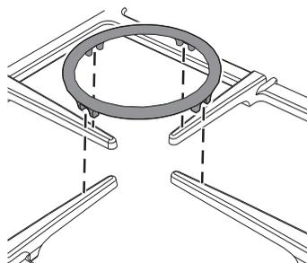
he pan support must be placed on the hob grid as shown in the figure above.
