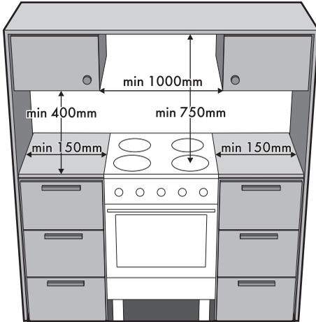
If a hood is installed above the hob, refer to the hood instruction manual to ensure the correct clearance is left.
