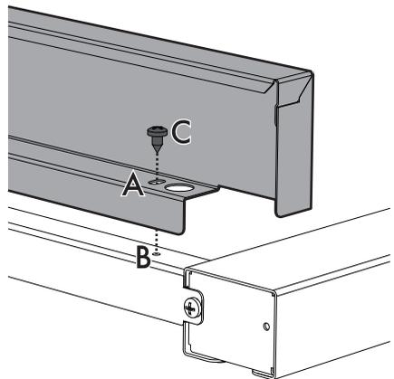
2. Secure the upstand to the top by tightening screws **C**.
