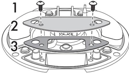
3. Replace the nozzle using a 7 mm spanner according to the gas to be used.
