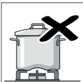
Do not use damaged pans, which do not sit evenly on the hob. Pans may tip over. Only use pans with a thick, flat base.
