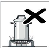
Use pans which are the right size for each burner. Do not use small pans on large burners. The flame must not touch the sides of the pan.
