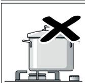
Always centre the pan over the burner, not to one side. Otherwise it could tip over. Do not place large pans on the burners near the control knobs. These may be damaged by the very high temperatures.
