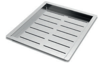
Stainless steel draining tray AISI 304 18/10 Stainless steel draining tray 1 mm thickness. Ext dimension: 370 x 440 mm Int dimension: 325 x 390 mm Depth: 30 mm
